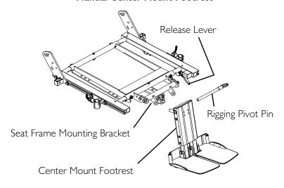
FIGURE 6.15 Removing/Installing the Center Mount Footrest
